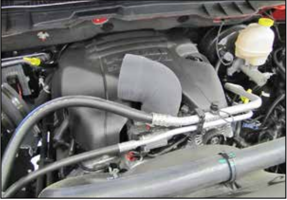
21. Install the provided silicone hose (084086-1) onto the throttle body and secure with the provided hose clamp. NOTE: Do not completely tighten at this time.
