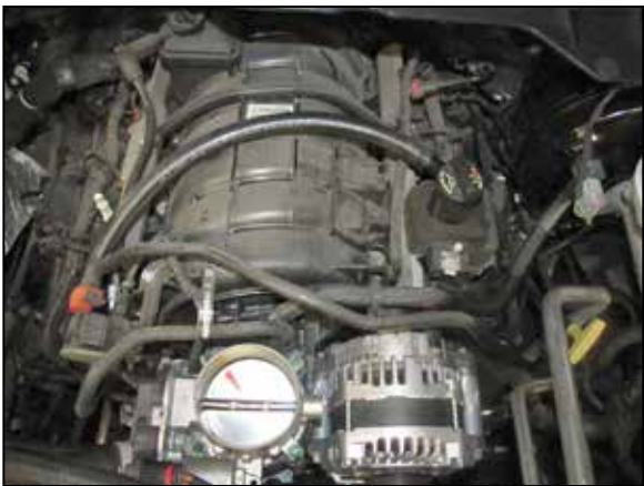
9. Install the K&N® CCV hose assembly onto the factory port and position the assembly as shown.
