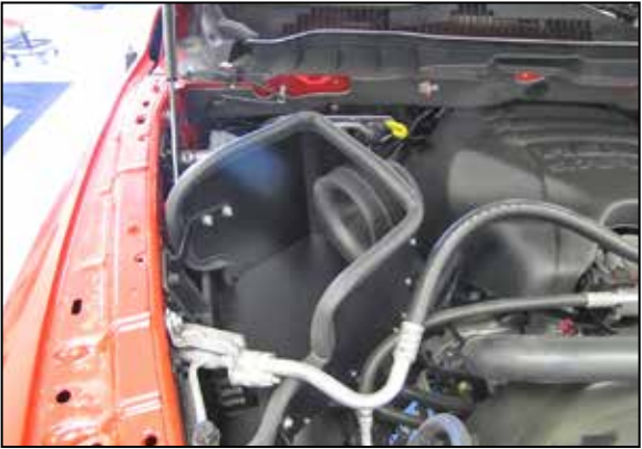
20. Install the heat shield into the vehicle and secure with the factory bolts from steps #18 and #19. NOTE: Do not completely tighten at this time.
