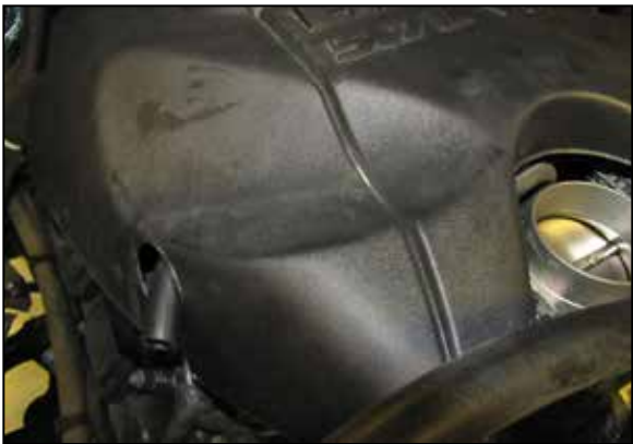
10. Reinstall the engine cover and position the CCV hose through the opening.
